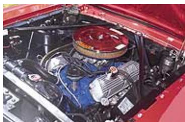
Besides the terrific original color, the red ride was outfitted with an A-code four-barrel 289 V-8 for power. This represents a considerable upgrade in power over the C-code two-barrel or base six-cylinder engines. The engine in Carl's rig was freshened up for the refurbishment with a complete rebuild. It is backed by the venerable C-4 three-speed Cruise-O-Matic transmission.
