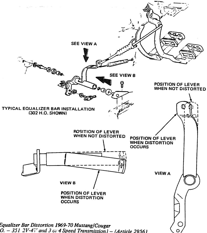
Figure 6 - Clutch Equalizer Bar Distortion 1969-70 Mustang/Cougar (302 H.O. - 351 2V-4V and 3 or 4 Speed Transmission) - (Article 2956)
